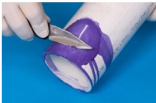
Using a knife or other sharp object, drag the edge over the coated surface. Proper penetration has been made if you can scratch or scrape a few thousandths of the primed surface away. Because weather conditions do affect priming and cementing action, repeated applications to both surfaces may be necessary. In cold weather more time is required for proper penetration.
