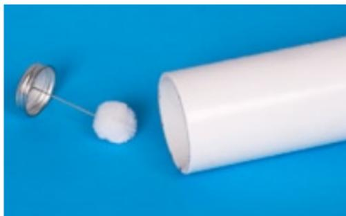
8. Priming; the purpose of a primer is to penetrate and soften the surfaces so they can fuse together. The proper use of a primer and checking its softening capability provides assurance that the surfaces are prepared for fusion in a wide variety of conditions. Check the penetration or softening on a piece of scrap pipe before you start the installation or if the weather changes during the day.
