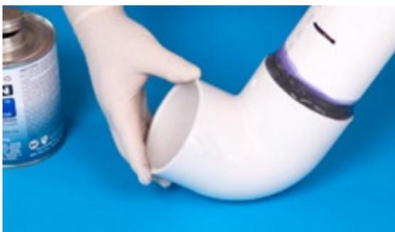
**19.** Using a rag, remove the excess cement from the pipe and fitting, including the ring or bead around the socket entrance, as it will needlessly soften the pipe and fitting, and does not add to joint strength. Excess cement around the socket entrance will also extend the cure time. Avoid disturbing or moving the joint.
