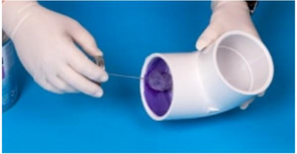
**10.** Next, aggressively apply the primer to the end of the pipe to a point 1/2" beyond the depth of the fitting socket.
