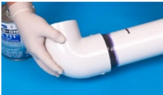
**18.** After assembly, a joint should have a ring or bead of cement completely around the juncture of the pipe and fitting. If voids (gaps) in this ring are present, sufficient cement was not applied and the joint may be defective.
