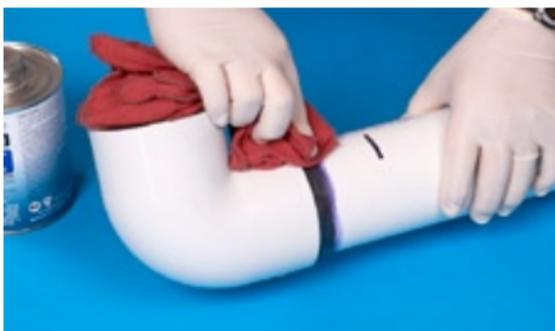
**20.** Handle newly assembled joints carefully until initial set has taken place. Follow IPS Weld-On set and cure times before handling or hydro-testing piping system (for set and cure times refer to page 22).
